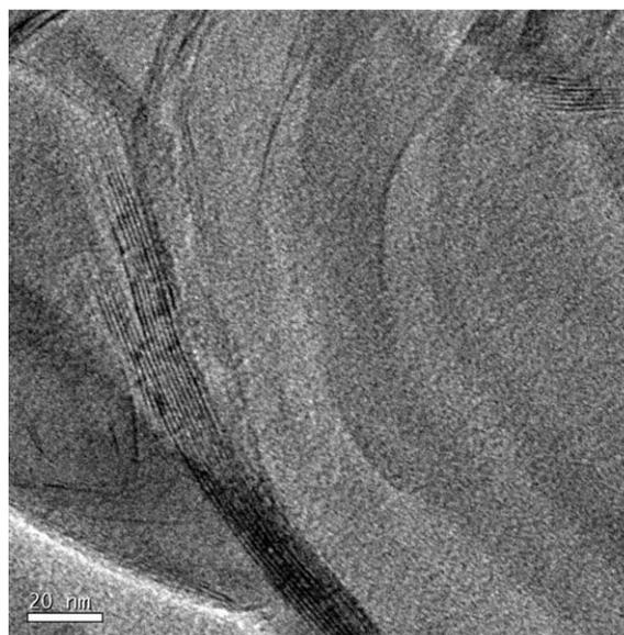
**Figure 8.** Agglomeration of Figure 7(a) for sample with  $\text{BF}_3\cdot\text{MEA}$  initiator, cured at  $100^\circ\text{C}$  for 2.5 h and postcured at  $180^\circ\text{C}$  for 1 h, viewed at higher magnification. Scale bar is 20 nm.
